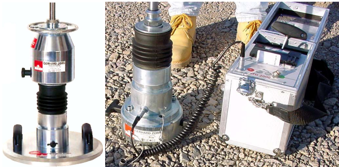
Figure 7: Alternative configurations of falling-weight deflectometer left: Medium-heavy falling-weight deflectometer using a 15 kg drop load and a load plate diameter of 300 mm.
