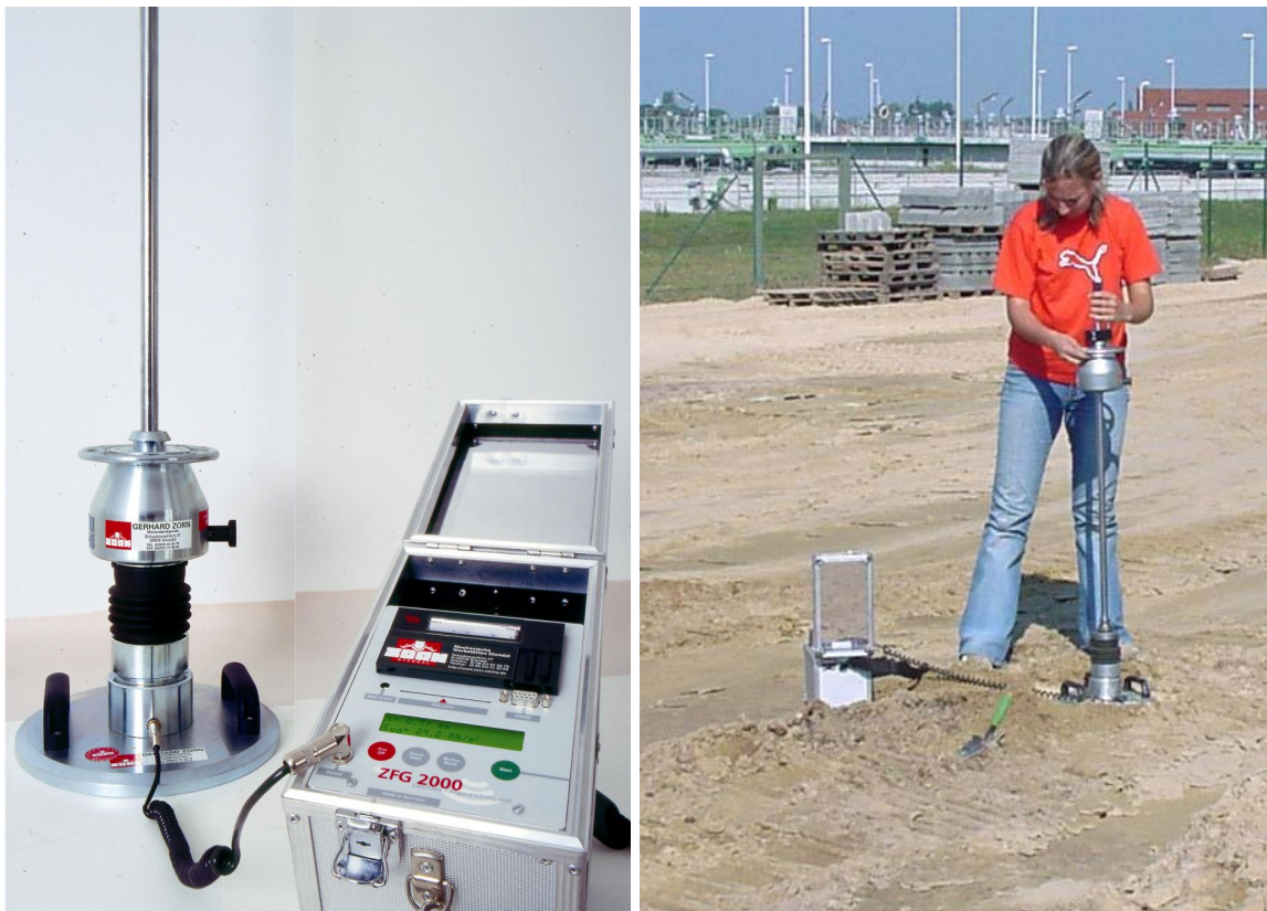
Figure 1: Dynamic plate load test using the Light-Weight Deflectometer according to TP BF-StB, Part B 8.3 left: ZFG 2000 test unit; right: single-person operation
